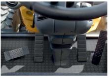
Manually switchable differential lock in front axle
