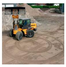
4.90 m turning radius measured over rear end
